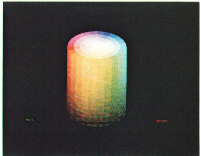
Fig. 2. Color cylinder model. Area-fill colors can be specified by selecting a point within this unit cylinder. The angle indicates the combination of red, blue, and green required, the radius specifies the amount of white, and the height corresponds to the luminosity.
